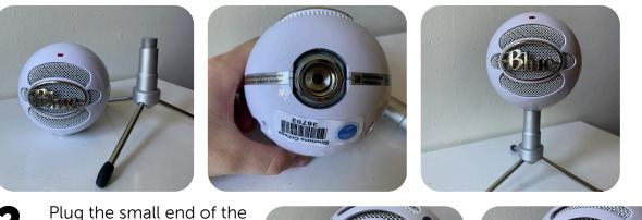
2 Plug the small end of the USB cord into the back of the microphone. Plug the other end of the USB into your computer.
